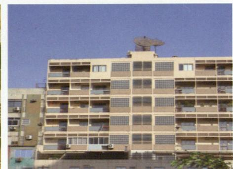
Walls and latticework / Walls with the extensive use of *brise-soleils*, continuous recessed windows with latticework and movable slate to block the sun and allow for ventilation. Balconies and terraces for seeing and being seen.
